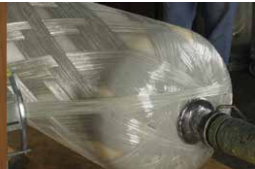
Miles of wound fiberglass sealed with epoxy resin over a polyethylene shell provide outstanding performance and durability.
